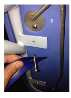
5) Place washer on screw, then screw through prepunched hole on one of the ends of the belt assembly. Washer <u>must</u> be applied as shown for each assembly.
