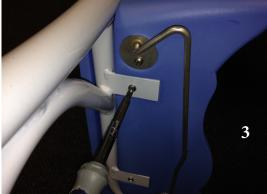
3) Remove seat screw as shown in picture 3.
