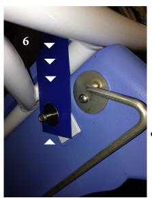
6) Run strap and screw through the frame arch identified in step one, then screw the completed assembly back onto seat bracket.
